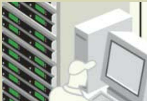
**The cell transmitter:** The transmitter allocates the programmes required to the antennas. The programmes are transmitted only once as files from the central PC to the various cell transmitters, where they are stored and fed to the antennas via a data cable.
